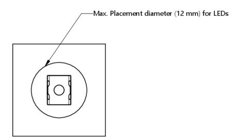
The maximum height of the LED must not exceed 2.4mm
