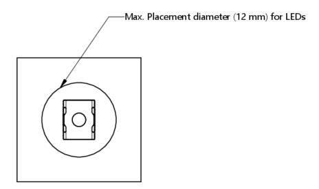
The maximum height of the LED must not exceed 2.4mm
