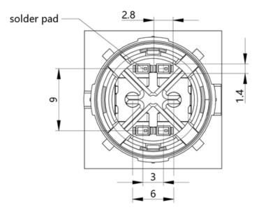
The maximum height of the LED must not exceed 2.4mm
