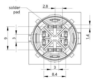
The maximum height of the LED must not exceed 2.4mm
